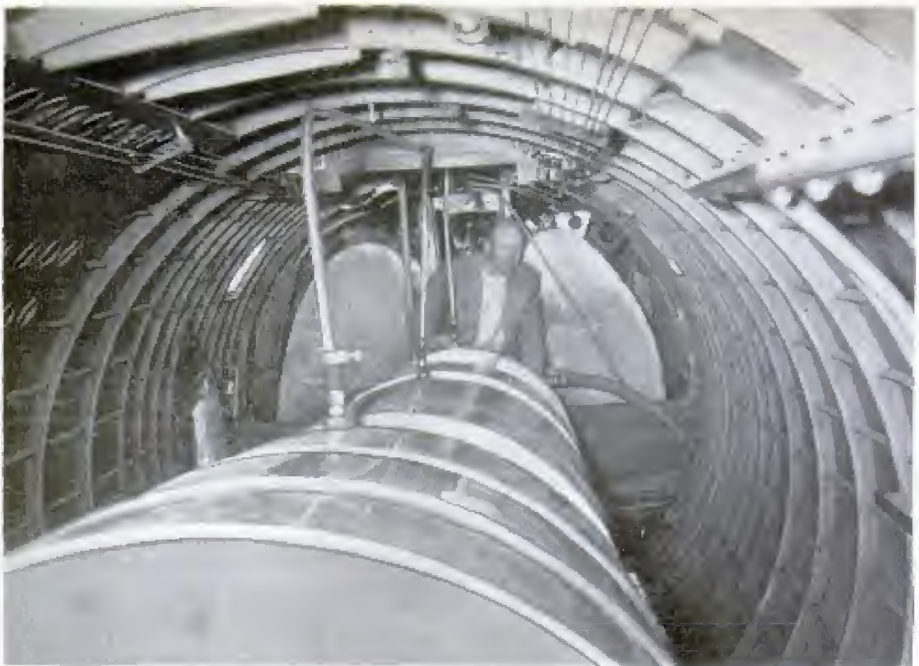
Built to carry bombs, the B-17's fuselage is almost filled by the eight interconnected insecticide tanks
